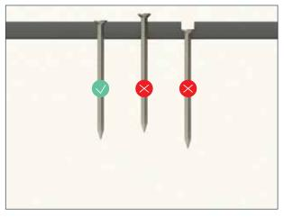
Do not countersink or angle fixings. Ensure fixings are proud of the surface of the plank.
