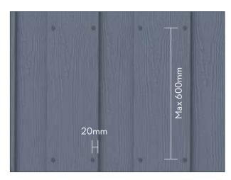
For visible fastening on timber battens, we recommend using Cembrit Facade Screw.
